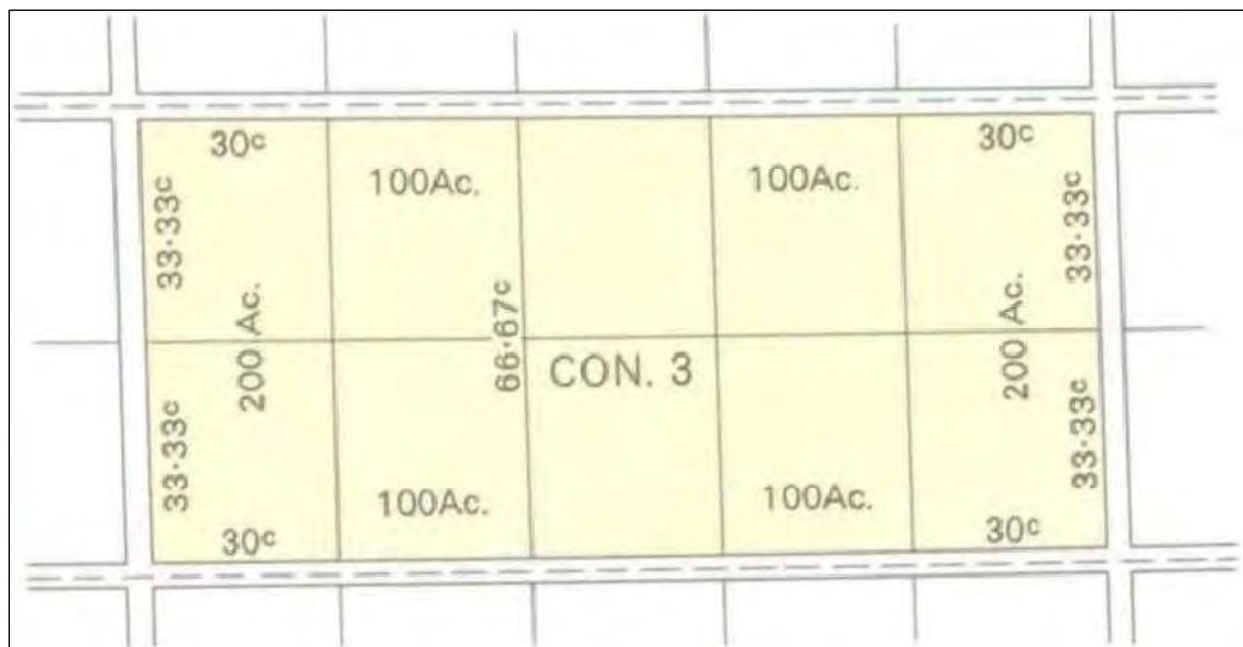
Plate 3: Double-Front Survey System (Dean 1969)
