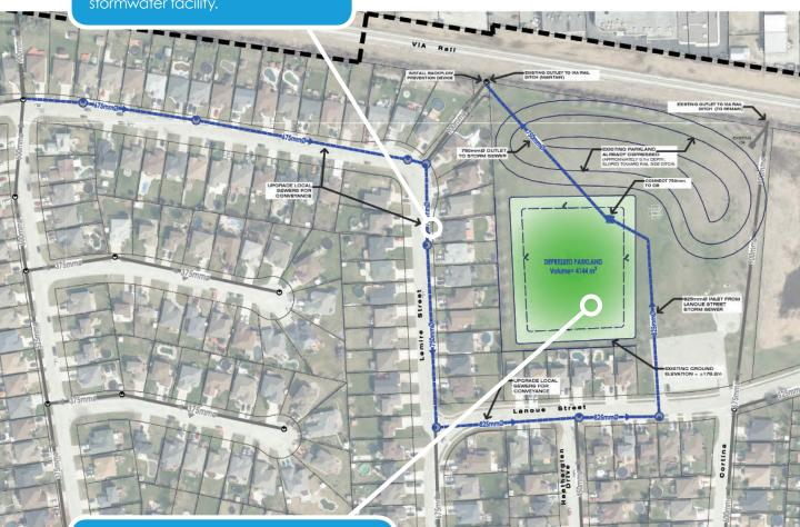
Depress southwestern portion of Buster Reaume Park by 0.80m to provide approximately 4,100 m3 of aboveground surface storage with a connection to the upgraded municipal storm sewers.
