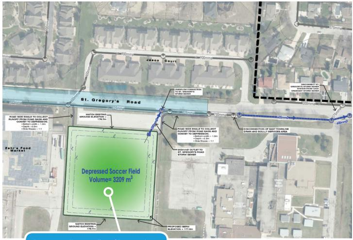
Depress northern portion of Tecumseh Soccer Fields Park by 0.70m to provide approximately 3,200 m³ of aboveground surface storage
