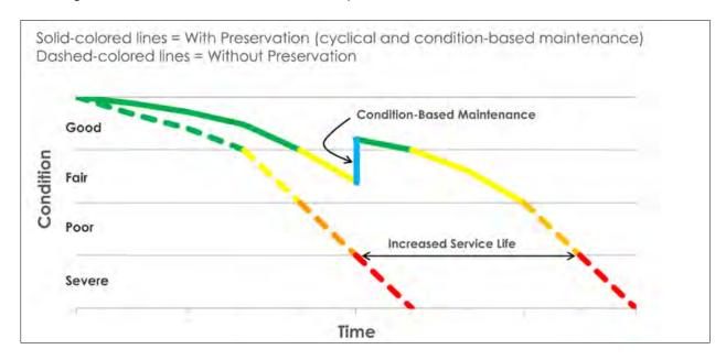
Figure 4-5: Smart Condition Based Maintenance Practices
