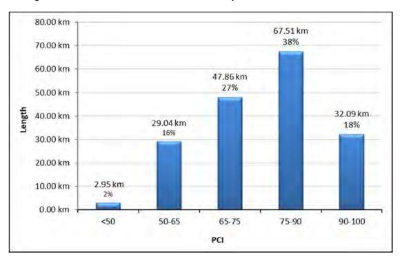
Figure 3-6: 2019 Pavement Condition Index (excludes Connecting Links)
