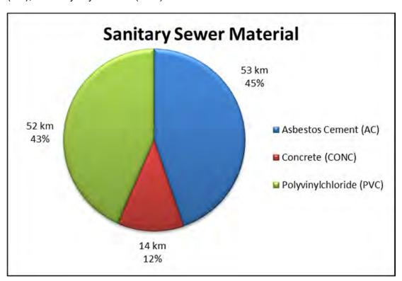
Figure 8-1: Sanitary Sewer Inventory by Material
