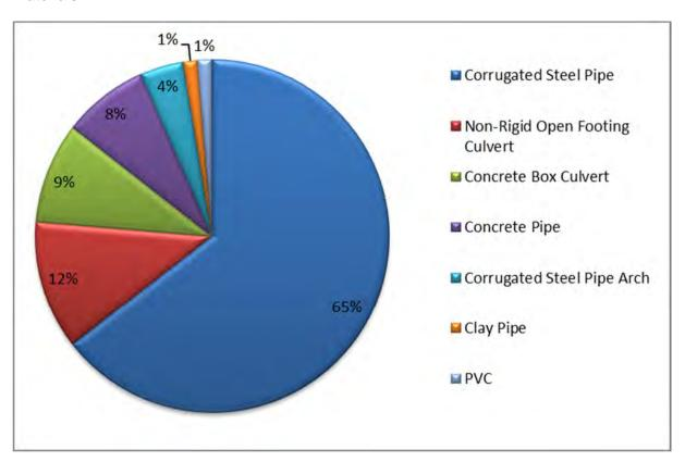
Figure 5-1: Culvert Types
