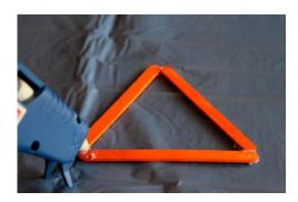
Step 3: Attach two more sticks to the first triangle. The two new sticks need to be glued to the corners of one side of the triangle. Two more sticks are glued to that triangle. Each new triangle should share a side with the previous triangle. Leave a gap at the center of your wheel, where the spokes meet up. Continue until your triangles meet up with the other side of the first triangle and you have created a wheel. Make a second wheel in the same manner.
