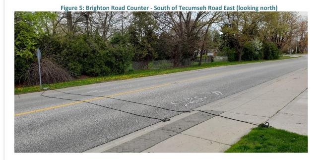
This pneumatic counter was mounted in front of 562 Brighton Road, approximately 25 metres north of the raised centre median's northerly limits.
